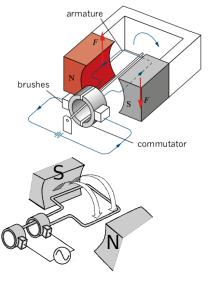
DC: split ring (two halves) AC: slip ring (separate rings with constant contact)
