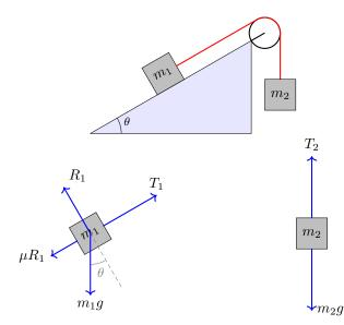
• **Suspended pulley:** tension in both sections of rope are equal
