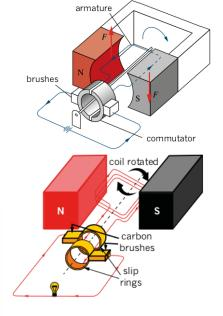
Force on I-carying wire, not Cu F = 0 for front back of coil (parallel) Any angle > 0 will produce force **DC:** split ring (two halves)
