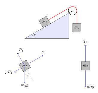
• Suspended pulley: tension in both sections of rope are equal  $|a| = g \frac{m_1 - m_2}{m_1 + m_2}$  where  $m_1$  accelerates down With tension:
