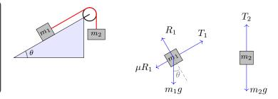
Suspended pulley: tension in both sections of rope are equal
